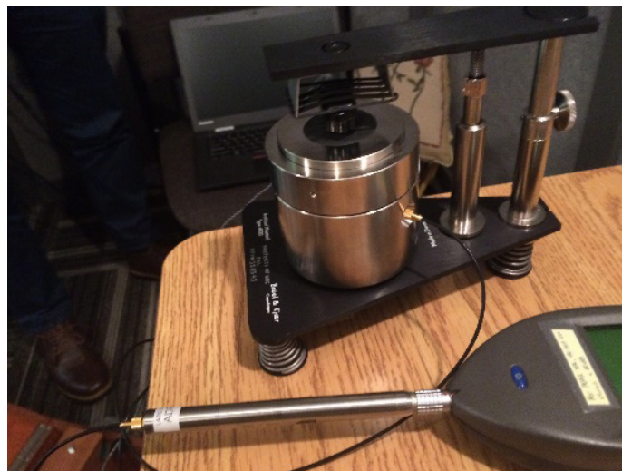
Figure 8: Example of appropriate equipment need for electroacoustic calibration: B&K 4930 artificial mastoid and Larson Davis sound level meter set up for bone-conduction calibration.
